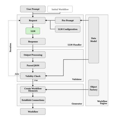
Figure 4.7: The proposed workflow with an integrated LLM, and LLM-handler (Reitenbach et al., 2024).
