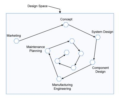
Figure 2.3: Point-based engineering explained (Toche et al., 2020).
