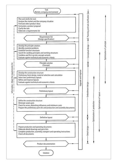
Figure 2.1: The ED process according to (Beitz et al., 1996)
