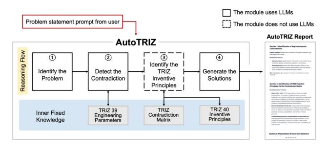
Figure 4.3: The process flow in AutoTRIZ (S. Jiang & Luo, 2024).
