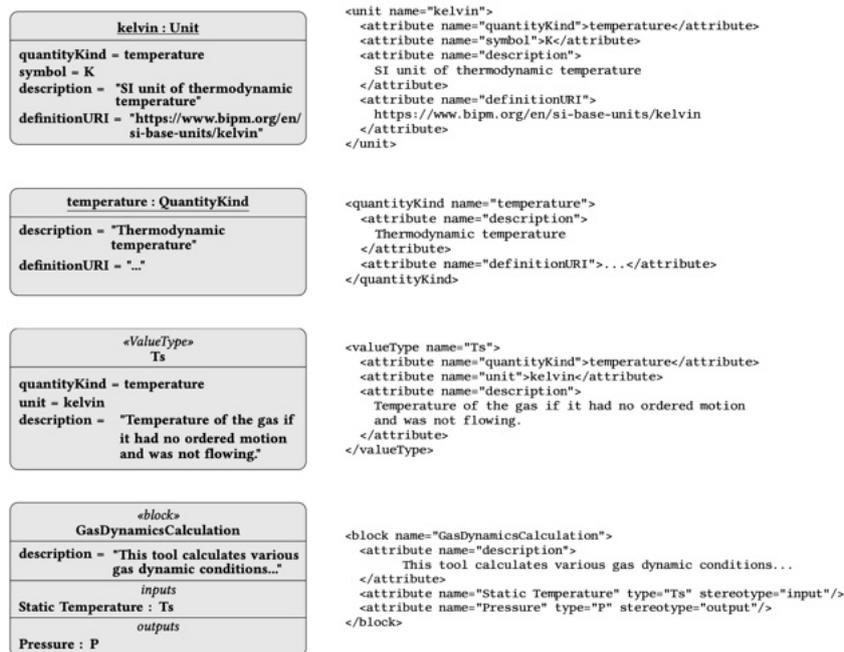
Fig. 2 SysML Serialization to XML-Format
